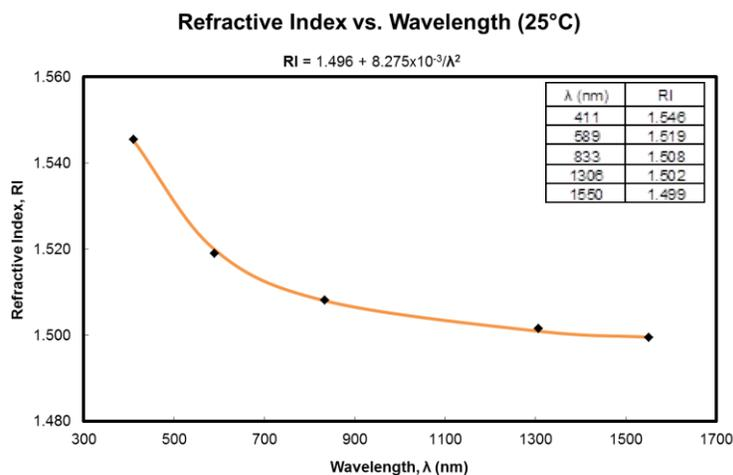
Figure 2. Refractive Index vs. Wavelength, at 25°C
