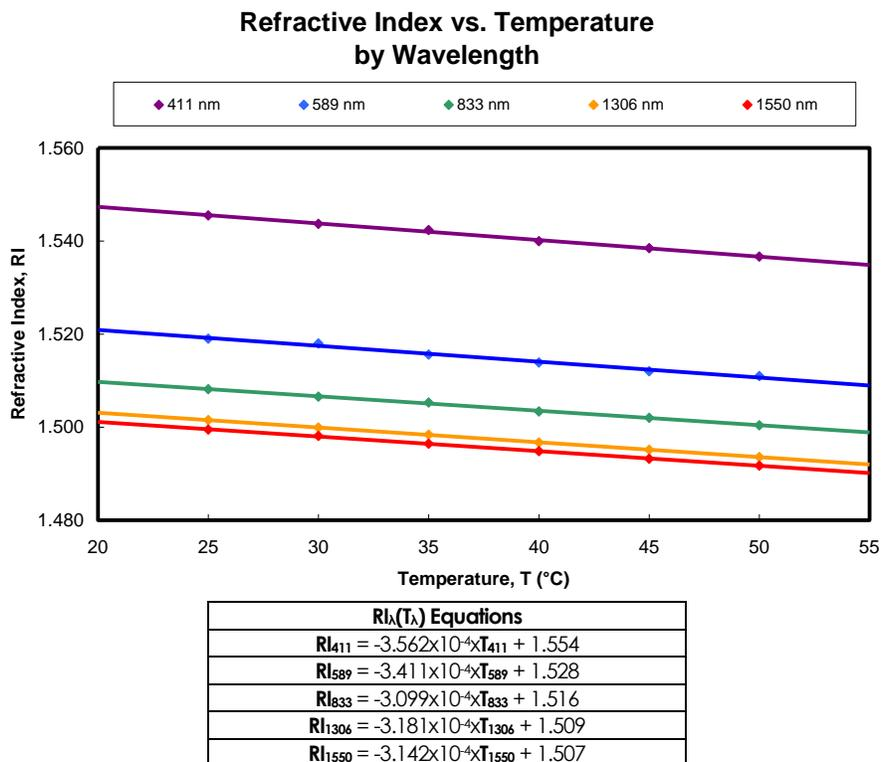
Figure 3. Refractive Index vs. Temperature, at various wavelengths.
